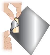
**2.** Roll the tube up in the foil on the table.
